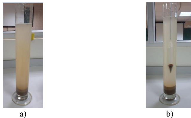
Fig. 2. Test process: a) soil before the hydrometer measurement; b) during the measurement process with hydrometer
