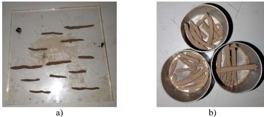
Fig. 5 The process of rolling the soil into flagella: a) at the rolling boundary; b) after drying in an oven
