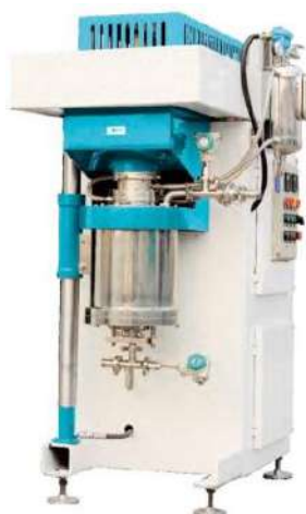
Figure 2. Rucca M bead mill with finger type rotor
